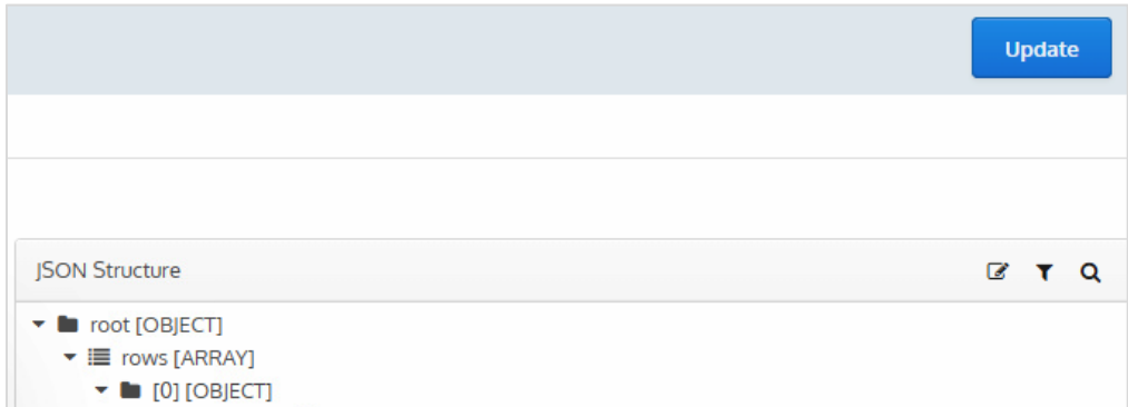
Figure 7 · Click Update to save the REST Monitor configuration and activate the new Metric Producer.
